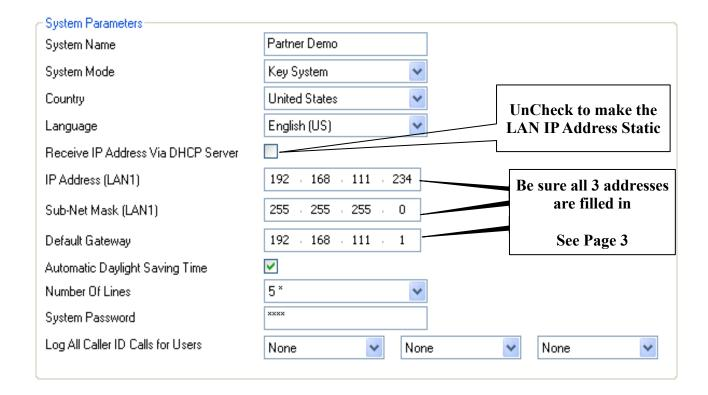
The KSU will obtain and display a LAN IP Address and Subnet Mask automatically.
